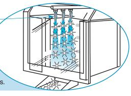
Airmiser nozzle cooling a hot spot in a plastic mould.
