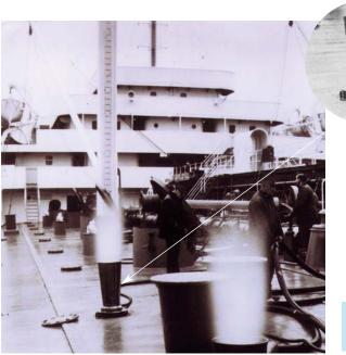
An EV8 extractor ventilator used to vent the cargo hold of a ship prior to cleaning.
