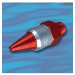
Material: Aluminium. Weight: 0.025kg dB(A) at: 5.5 bar is 83 Inlet Thread:  $G_4^1$
