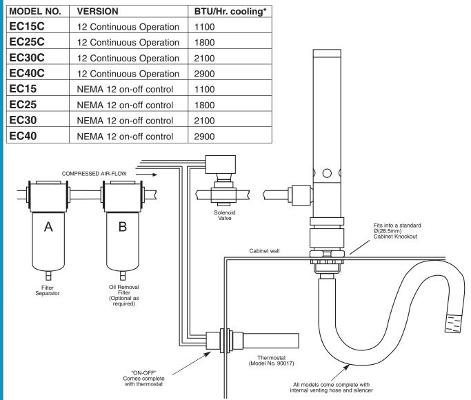
ALL 'CONTINUOUS" OPERATING MODELS INCLUDE: COLD AIR INTERNAL VENTING HOSE & SILENCER ALL "ON-OFF" OPERATING MODELS INCLUDE:
